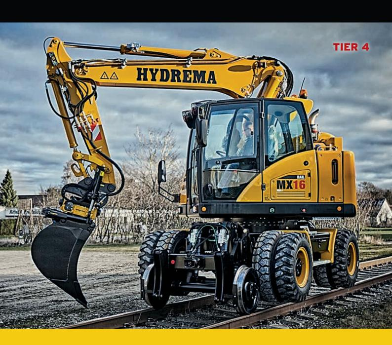
Specially designed compact excavator in the 19 tonne class for railway work with focus on great stability, high performance and flexibility.
